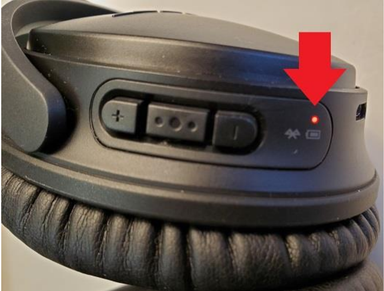
Figure 34 - Blinking Red: Charge Immediately
